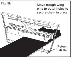
**STEP 10. Lift the Belt.** Turn the Adjusting Nut counterclockwise until the belt is at the desired height. (Use the correct size socket and tool—not included.) Remove the ratchet or power tool prior to starting work.
