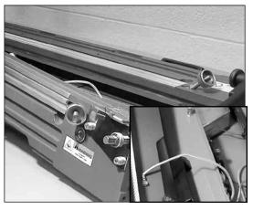
**4.** Swing control end platen side out of front plate retention grooves. Place platen near machine. **Caution!** A ground wire is attached to the fixed platen. Use caution to avoid damage to this wire and connection.
