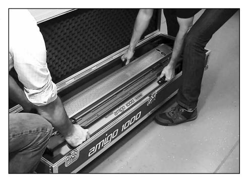
Open transport case and lift machine from case. **Caution!** Two persons required to lift and place machine. Position machine on even surface with platens up and level. Do NOT apply power until belt is cut and clamped in preparation for splicing. Ensure power inlet, controls, and cutter crank are accessible.
