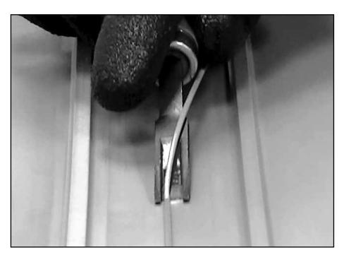
Remove underside weld bead with skiving tool.
