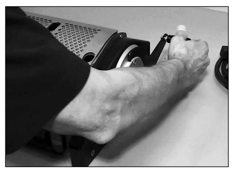
Rotate actuating lever to its operating position.
