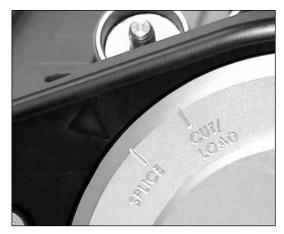
1. Rotate actuator lever to SPLICE position. **Caution!** Emitter is exposed during operation. Use caution to avoid damage.
