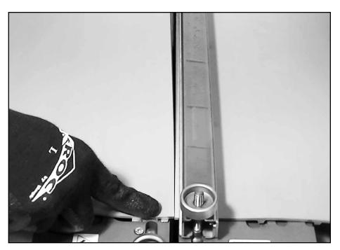
Load belt ends, aligning edges of prepared belt.
