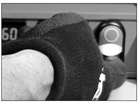
When machine cools to "splice start" temperature and light illuminates, immediately press green start button to initiate splice heating cycle. Closely attend machine during splice cycle.
