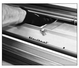
**7.** Raise emitter to access beneath sliding platen for cleaning opposite side. Lower emitter after cleaning.
