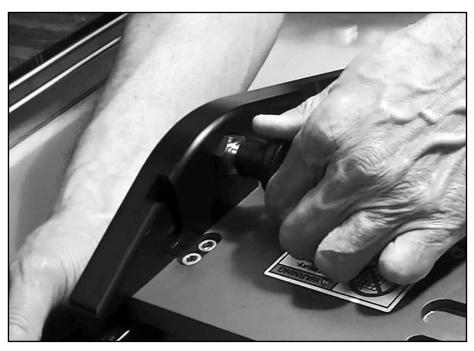
Lock in place with locking pin.
