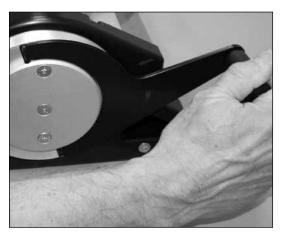
6. Rotate actuator lever/cam disk to close platens.
