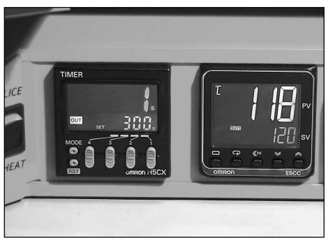
Allow preheat period to expire. A sound tone will be heard at conclusion of preheat cycle. Allow machine and belt to cool to preset "splice start" temperature.
