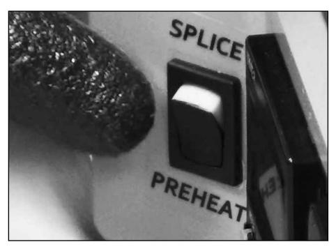
Place heating mode switch to PREHEAT position.
