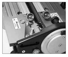
**2.** Slide fixed platen back in front plate retention grooves.
