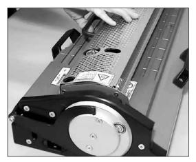
**10.** Install guard and operate 3 to 5, 70-second cycles on splice setting. Allow emitter to cool between cycles.
