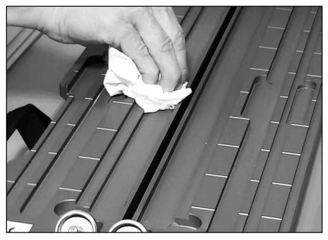
Ensure template and platen receiving slots are clean and debris-free.
