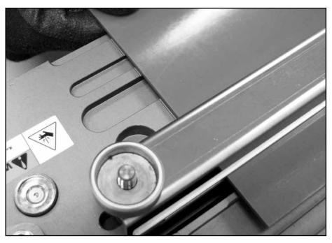
Ensure belt is positioned "square" to machine by either engagement of positive drive feature, or by using a square or alignment marks. **Note!** Belt widths less than 760 mm (30") should be centered in machine for splicing.
